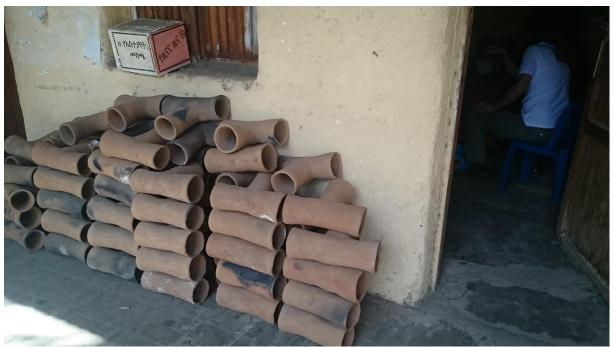
The outlets, which are fixed outside of the house wall, are made from fired clay
