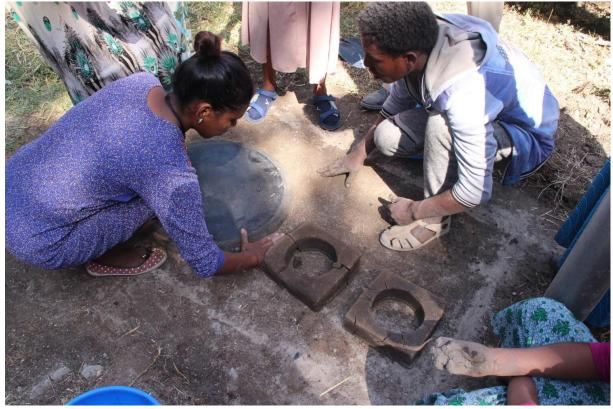
The chimney-bricks are air-dried, not fired
