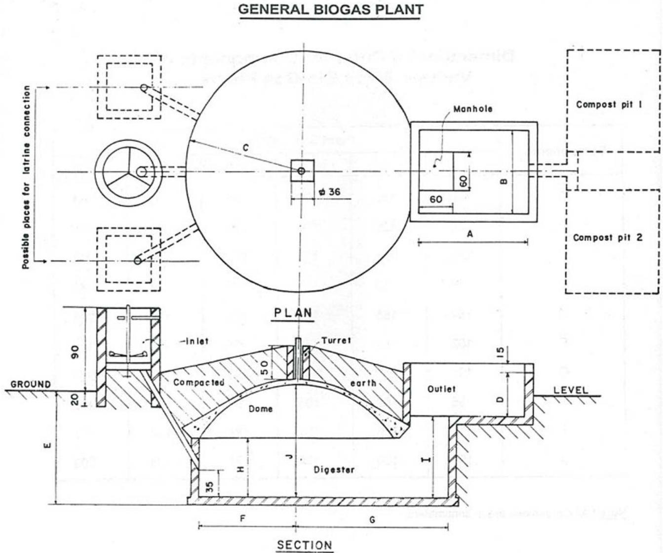
Figure 6.1: GGC 2047 model biogas plant
