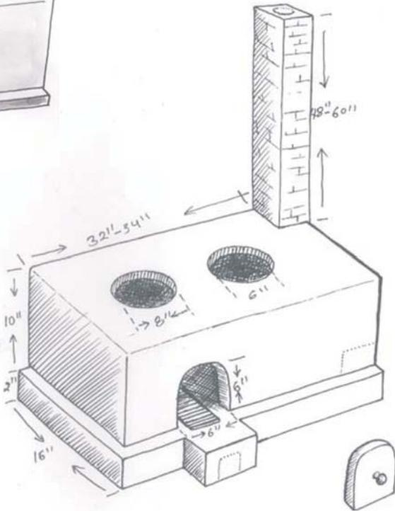
Figure 3.5 Two potholes ICS with raised second pothole
