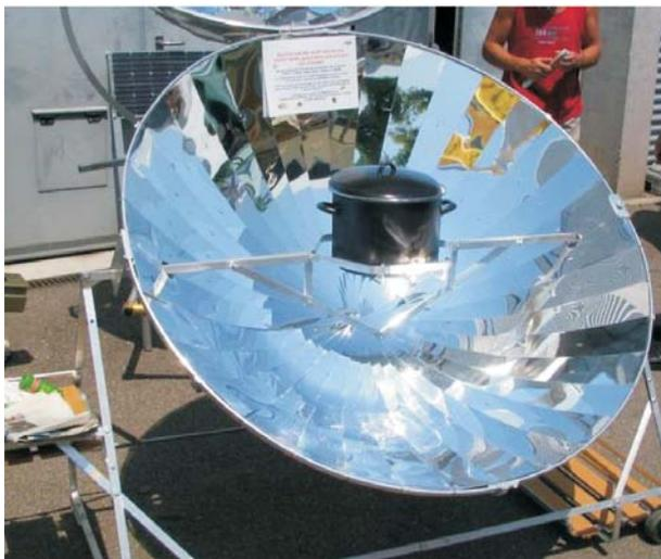
Parabolic type solar cooker
