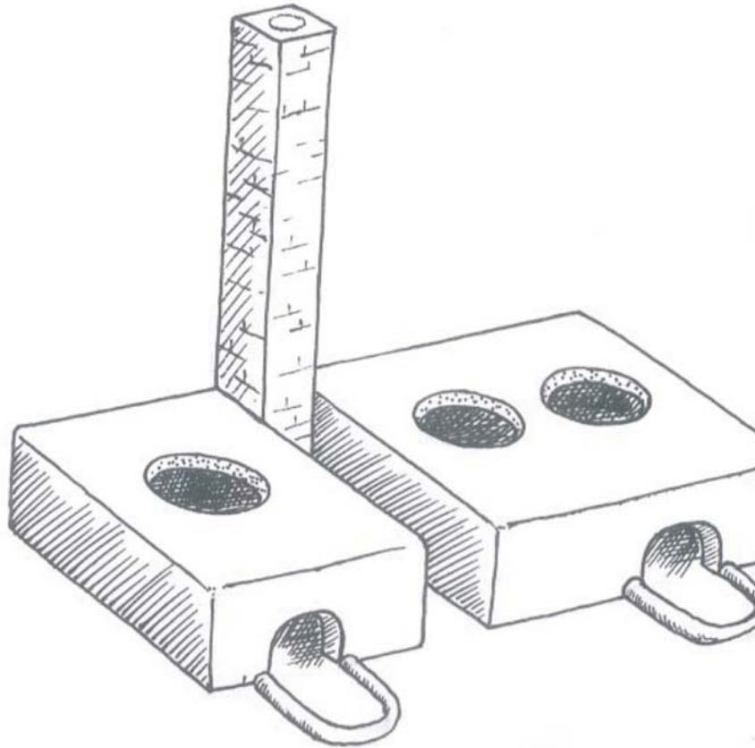
Figure 3.11: Three potholes multipurpose ICS
