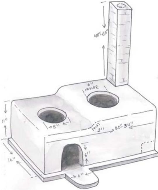
Figure 3.6 Two potholes ICS with grate
